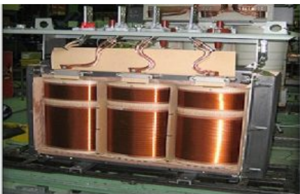
Fig.3 Amorphous metal transformer
