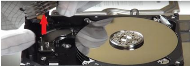
Fig.7. Removing the upper magnet.
