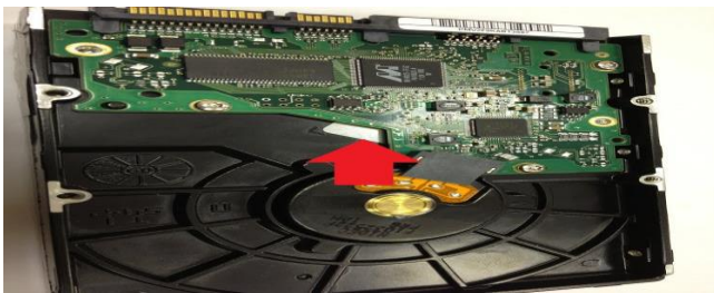
Fig. 3. Checking the status of the pads on the controller board.
