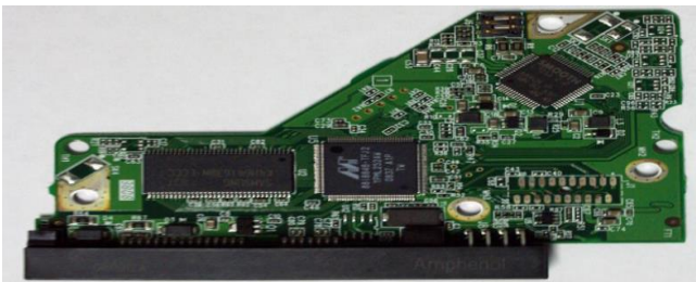
Fig. 4. Contacts connecting the controller board to the magnetic head unit (HSA).
